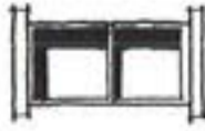
Double Hung Window Characteristics of: • All styles except Art Moderne • International Style
